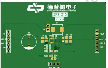
**1.** The feedback network, resistor R1 and R2, should be kept close to FB pin. Vout sense path should stay away from noisy nodes, such as SW & BS signals and preferably through a layer on the other side of shielding layer.
