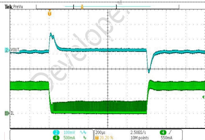
Load Step 0.1 to 0.9A, 1A/us Slew rate
